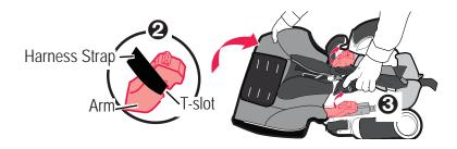
3. Arms should CLICK into the gutters. Seat assembly should appear as shown **4**.
